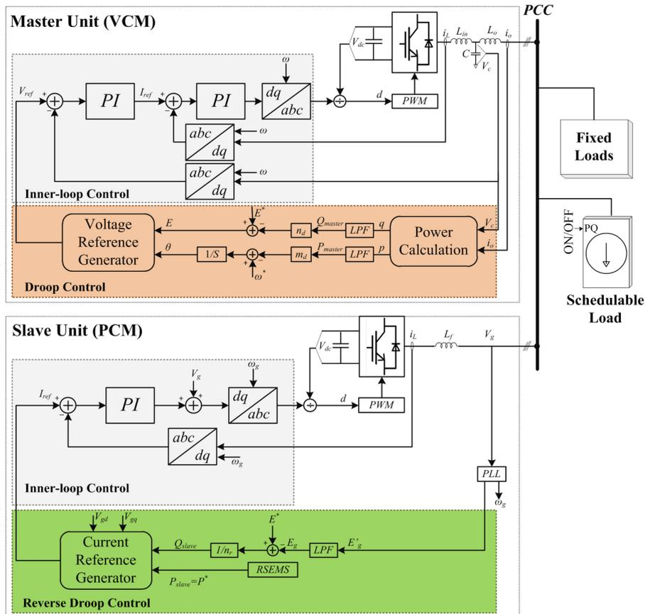
**Fig. 3** Master-slave control of distributed energy sources
