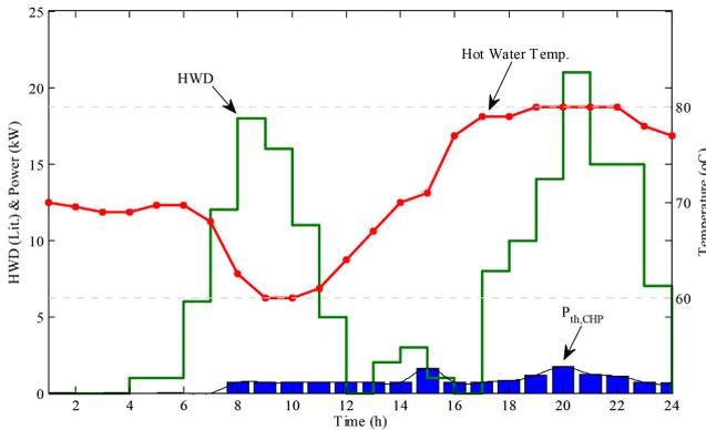
**Fig. 8** Operation of the  $\mu$ CHP based on the hourly hot water demand
